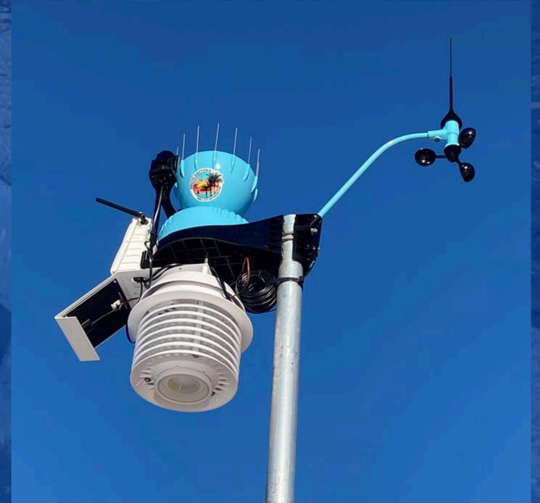
The City has installed a weather station atop City Hall that measures atmospheric conditions which will be used to document our stormwater system's performance compared to measured rain events.
