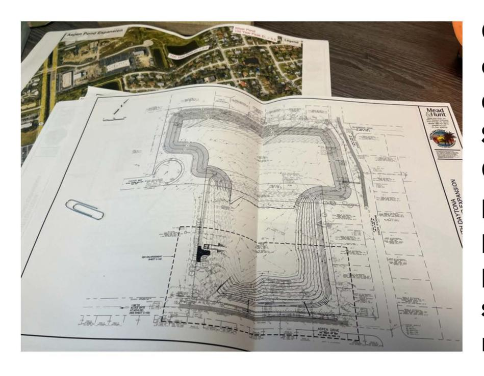
City staff recently met with project engineers to review the preliminary plans for the design Aspen Stormwater Pond Expansion Project. One of the key features being proposed is the addition of a second pump station, which will enhance pumping capacity and ensure greater system reliability through built-in redundancy.
