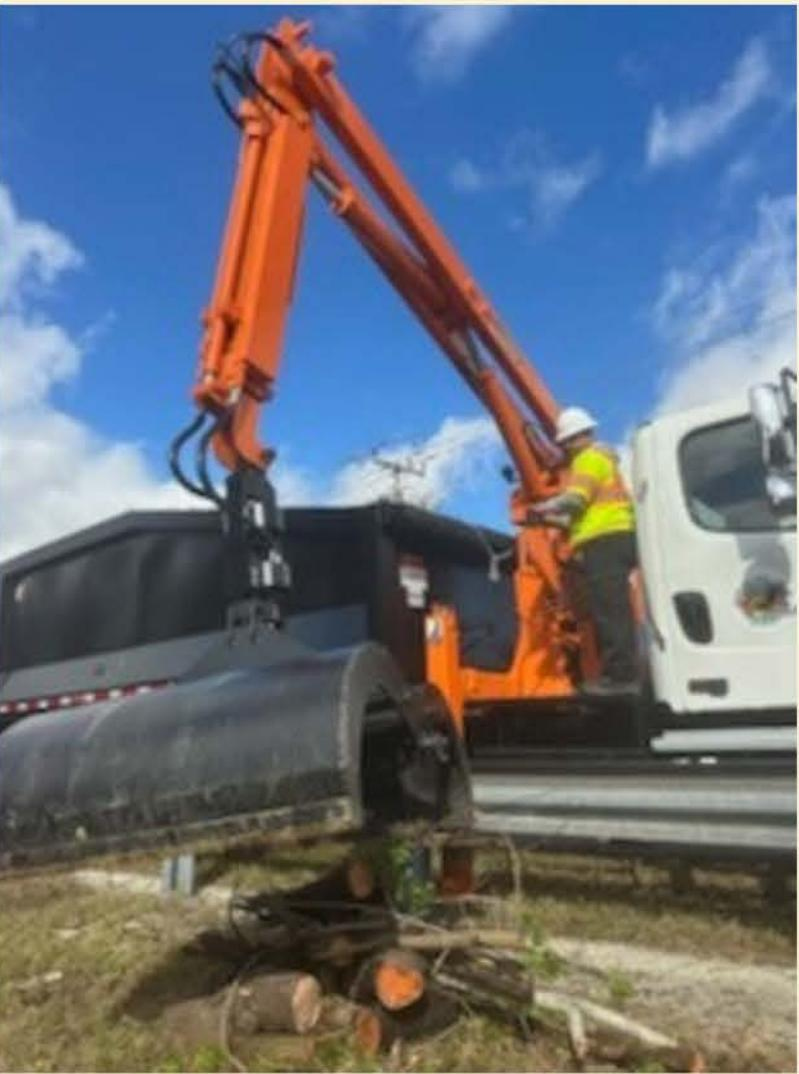
**Public Works Crews were excited to put the new claw truck to work on Reed Canal. Crews cleared brush along the canal and used the new truck to efficiently remove brush piles, improving access and overall conditions in the area.**
