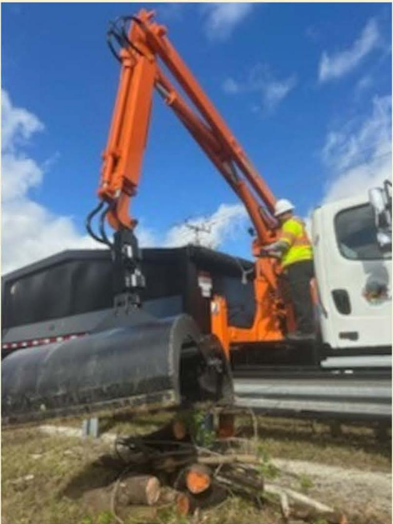
Public Works crews put the City's new claw truck to work along Reed Canal. Crews cleared brush and efficiently removed debris piles, helping stormwater flow more freely through the canal.
