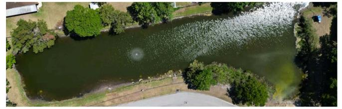
City crews have begun work on expanding Silver Pond in Big Tree Village. This project will increase stormwater capacity, helping to improve drainage and reduce flooding in the area.
