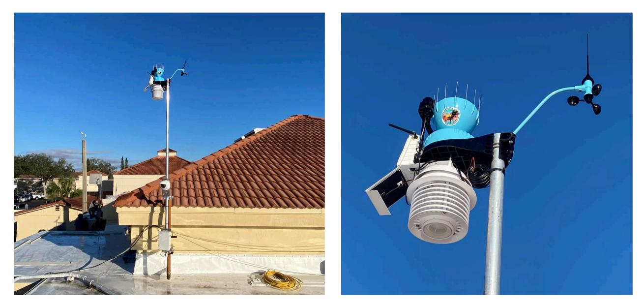
The City has installed a weather station atop City Hall that measures atmospheric conditions which will be used to document our stormwater system's performance compared to measured rain events.
