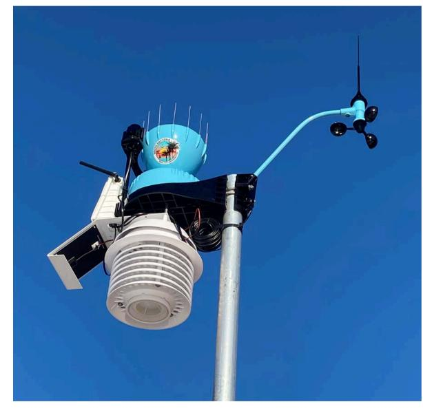
The City has installed a weather station atop City Hall that measures atmospheric conditions which will be used to document our stormwater system's performance compared to measured rain events.
